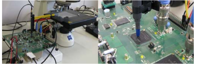
Fig. 2: Stepper table, SASEBO-G, and HF near-field probe
